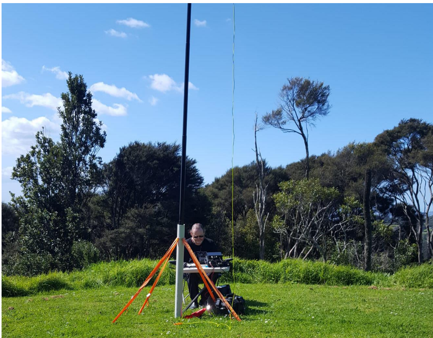
Glenn ZL1MY operating a Parks on the Air (POTA) station from the Waitkaere Ranges, near Auckland. He is using a Yaseu FT-897D powered by a deep-cycle marine battery, the pole is a 12m Spiderbeam fibreglass pole which supports a linked dipole.
