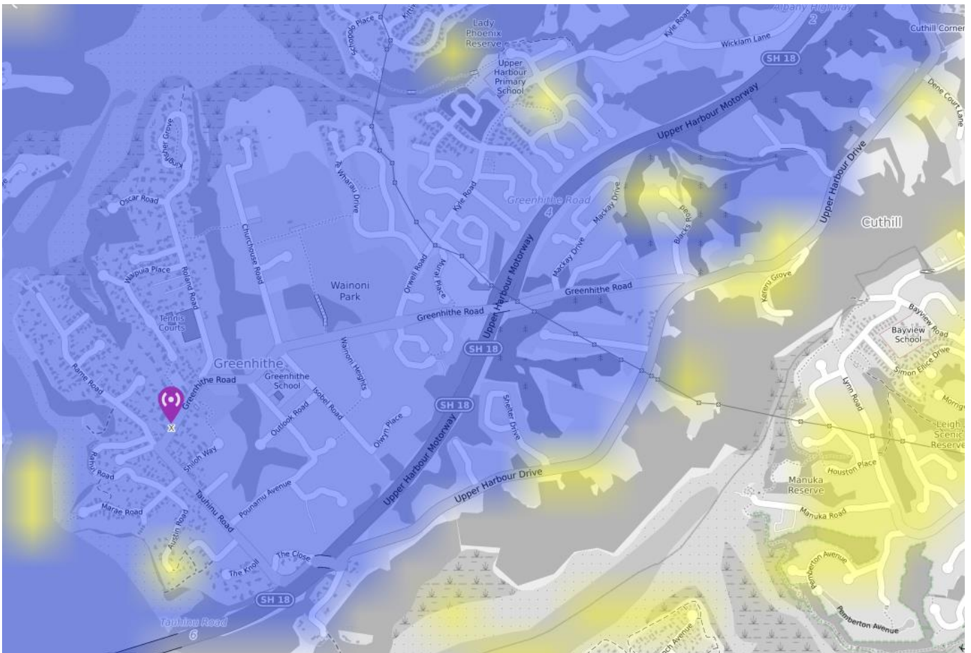
Above: Radio Mobile map showing predicted coverage around Greenhithe using 5-watt PRS radios and a base antenna at 1.5m above ground level.
