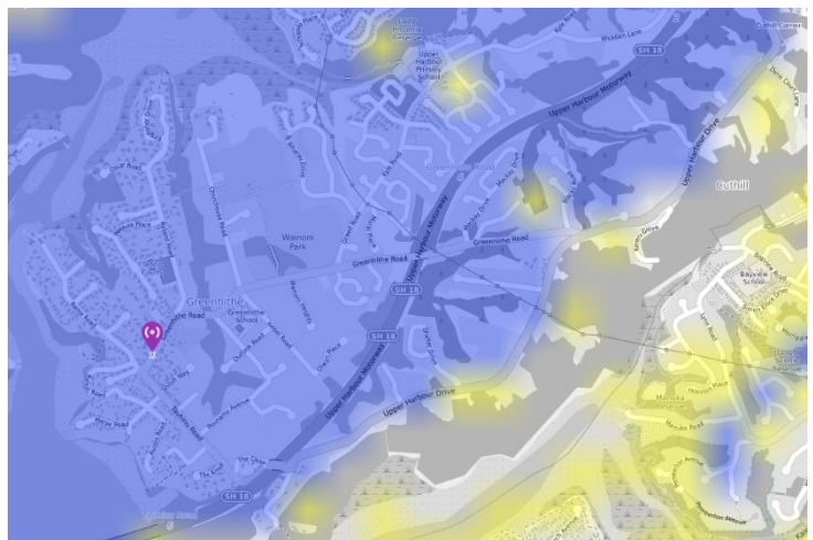
Above: Predicted coverage Greenhithe – PRS 5-watts. Base antenna 8m AGL
