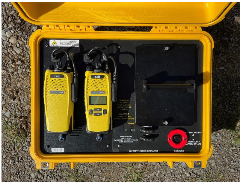
Left: Also at Dip Flat was the new Police SAR repeater manufactured by Tait. This includes two TP9300 series radios, lithium battery and charging circuitry, duplexer and interfaces.
